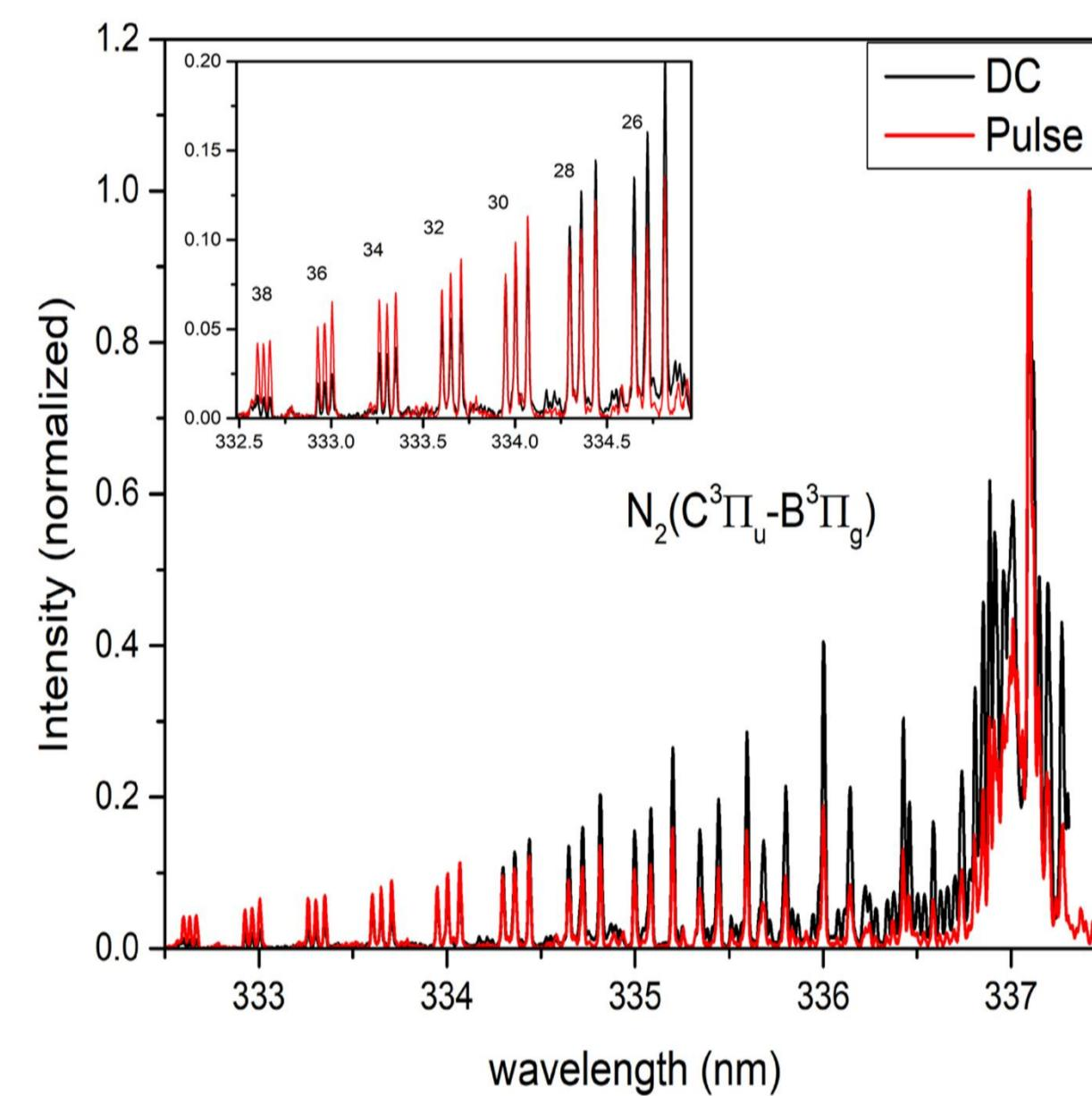
**Figure 4.** The comparison between  $N_2(C^3\Pi_u - B^3\Pi_g)$  band recorded in the second order of diffraction grating during pulsed and DC regime. The enlarged part of spectrum showing  $R_2$  branch lines with  $J=26-38$  is given in the inset. Experimental conditions: pulse width of  $800 \mu\text{s}$ , duty cycle of 5 %, gap of 2.5 mm,  $I = 20 \text{ mA}$ ,  $U_{\text{PULS}} = 460 \text{ V}$  ( $U_{\text{DC}} = 1500 \text{ V}$ ).
