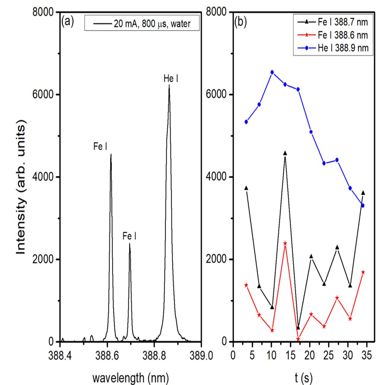
**Figure 7.** The Fe I and He I lines in the range of  $388.4$ - $389 \text{ nm}$ : (a) the intensity alteration during time period of  $0$ - $35 \text{ s}$  (CCD acquisition time 3400 ms). Experimental conditions: water drop treatment, pulse width of  $800 \mu\text{s}$ , duty cycle of 5 %, overall gap of 3 mm,  $I = 20 \text{ mA}$ ,  $U_{\text{START}} = 800$ - $1000 \text{ V}$ ,  $U_{\text{STABLE}} = 550 \text{ V}$ .
