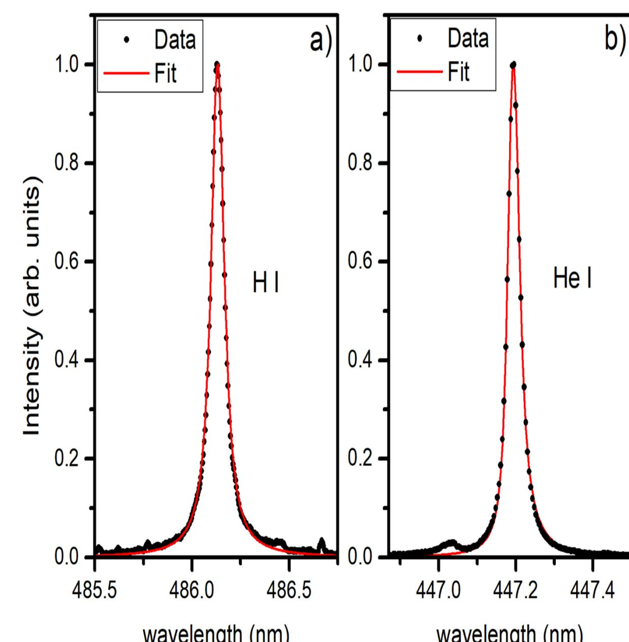
**Figure 5.** The best fit of (a) the  $H_\beta$  and (b) He I 447.2 nm line profiles recorded in the second order of diffraction grating. Experimental conditions: pulse width of  $800 \mu\text{s}$ , duty cycle of 5 %, gap of 2 mm,  $I = 20 \text{ mA}$ ,  $U_{\text{PULS}} = 434 \text{ V}$  ( $U_{\text{DC}} = 1500 \text{ V}$ ).
