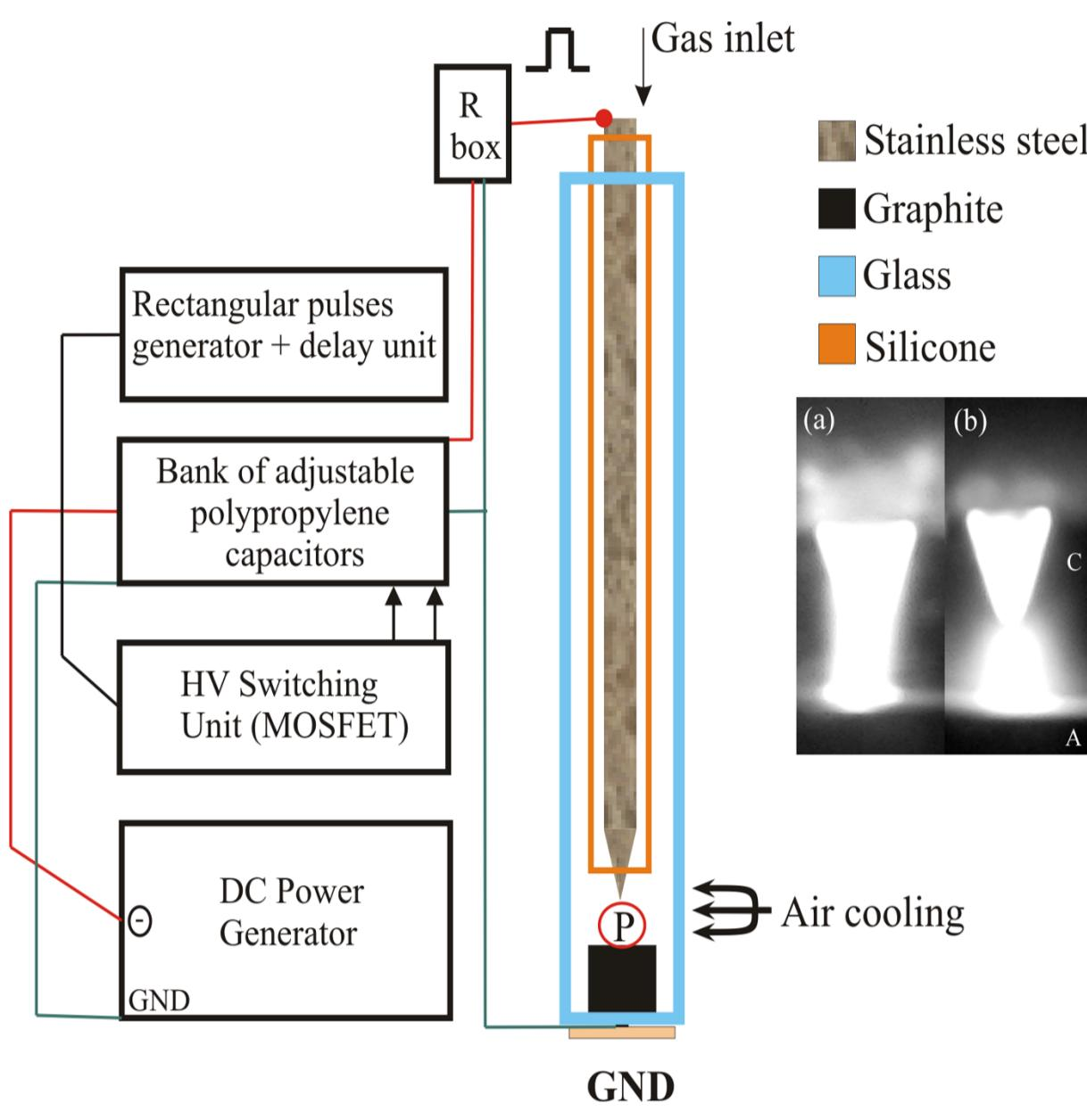
**Figure 1.** The schematic description of pulsed voltage generator and the cross section of atmospheric pressure gas discharge source. The photos of discharge burning in pulsed (a) and (b) DC regime are given in the inset.
