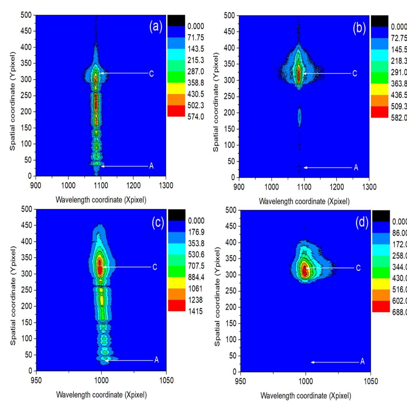
**Figure 3.** The  $H_\beta$  line in pulsed (a) and DC regime (b) and He I 447.2 nm line in pulsed (c) and DC regime (d) recorded by means of CCD camera imaging mode. Experimental conditions: pulse width of  $800 \mu\text{s}$ , duty cycle of 5 %, gap of 2 mm,  $I = 20 \text{ mA}$ ,  $U_{\text{PULS}} = 435 \text{ V}$  ( $U_{\text{DC}} = 1500 \text{ V}$ ).
