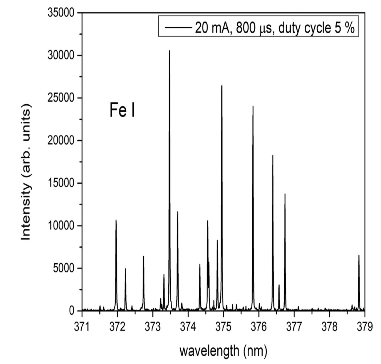
**Figure 6.** The spectrum of Fe I lines in the range of  $371$ - $379 \text{ nm}$  ( $I = 20 \text{ mA}$  and pulse width  $800 \mu\text{s}$ ). The diffraction grating operated in the second diffraction order.
