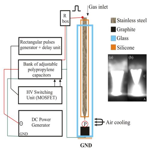
**Figure 1.** The schematic description of pulsed voltage generator and the cross section of atmospheric pressure gas discharge source. The photos of discharge burning in pulsed (a) and DC regime are given in the inset.
