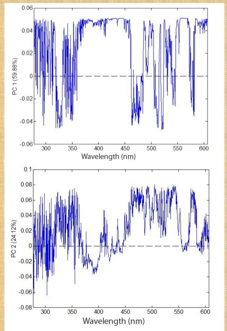
First two principal components of substrate LIBS data are shown above.
