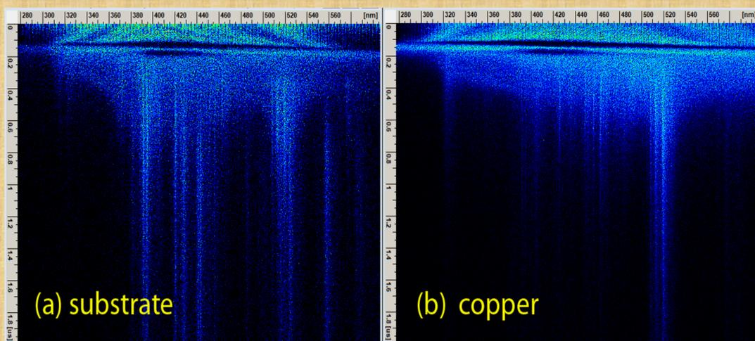
Streak images of plasma breakdown optical spectra of printed circuit board at the start, when only copper is ablated; and when the substrate is fully exposed, are shown above. Their differences could be seen by a naked eye.
