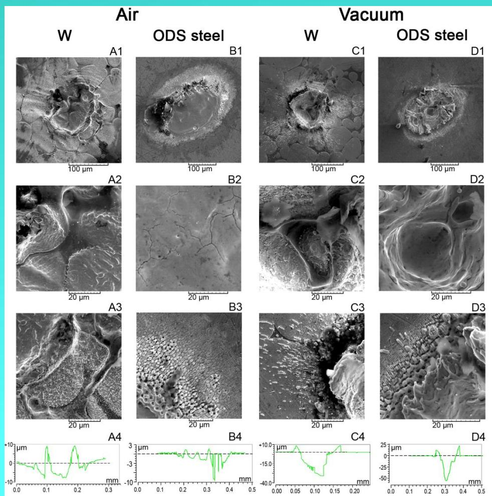
Laser pulse energy of  $\sim 5.2$  mJ, intensity  $10^{15}$  W/cm<sup>2</sup> (100 pulses), induced distinguishing surface features and phenomena. Generally, they are in strong correlation with sample type and ambience:
